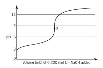
The graph shows the changes in pH that occur when 20.00 mL of 0.100 mol  $L^{-1}$  benzoic acid solution in a conical flask is titrated with 0.200 mol  $L^{-1}$  NaOH solution from a burette.
